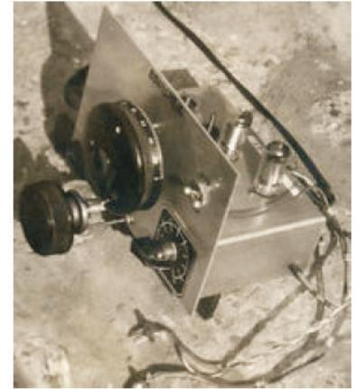
*a radio made using vacuum tubes*
