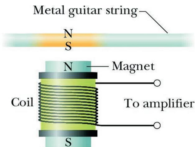
to **Pictorial representation of a single coil pickup (only one pole shown) at work**
