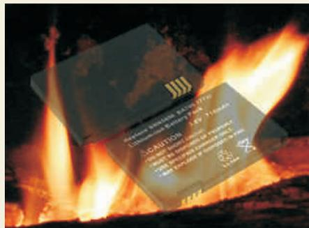
more than 2 billion batteries are produced a year for laptops, mobile phone, Digital cameras and many more. Steps are being taken by manufacturers to render them as the safest batteries, some are (1) protection to inhibit high current surges (2) Fuse to cut current flow if its temperature increases above a threshold (3) Fuse to prevent excessive charging or discharging of the battery . We can observe some
