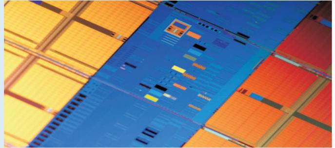
Close-up of a 45nm SRAM Test Wafer
