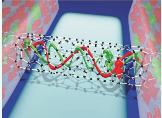
spin space in a spin heterostructure and the application of scheme in spintronic devices. Similar to the Josephson Effect, the equilibrium spin current is generated by the phase difference between the spin wave functions on the two sides of a junction. This problem is of important practical interest, because a spin current can be generated in a spin heterostructure without any external charge current and voltage and the approach has potential applications in low power spintronic devices.
